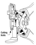
**Single Row Pairing Jacks:** Insert the 110 blade in the *lower* position of the holding fixture, with the cutting knife of the blade facing away from the tool.
