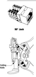
**90° Jacks:** Insert the 110 blade in the *lower* position of the holding fixture, with the cutting knife of the blade facing the tool.
